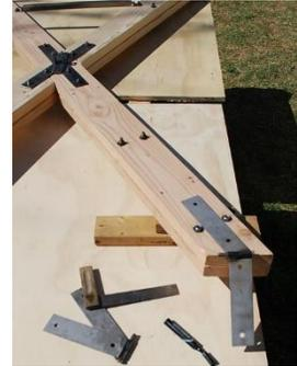
Step 31. Attach Part #1, the two-piece adjustable square tubing brace, to the bracket at the back center of the cross using a  $2\frac{1}{2}$ " Clevis Pin.
